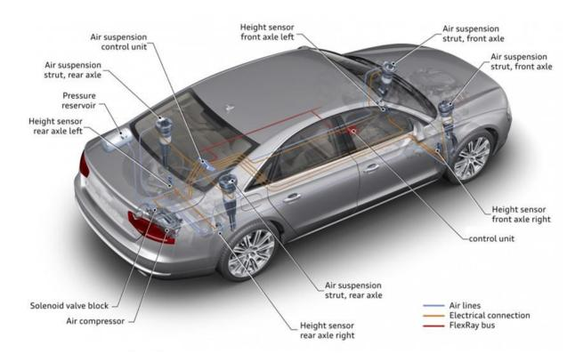
The suspension struts and shock absorbers of the air suspension system are similar to a conventional suspension system, but the metal coil springs are replaced by air springs. Nevertheless, the air spring does have different characteristics than a coil spring therefore the dampening setting of the shock is tuned differently.
